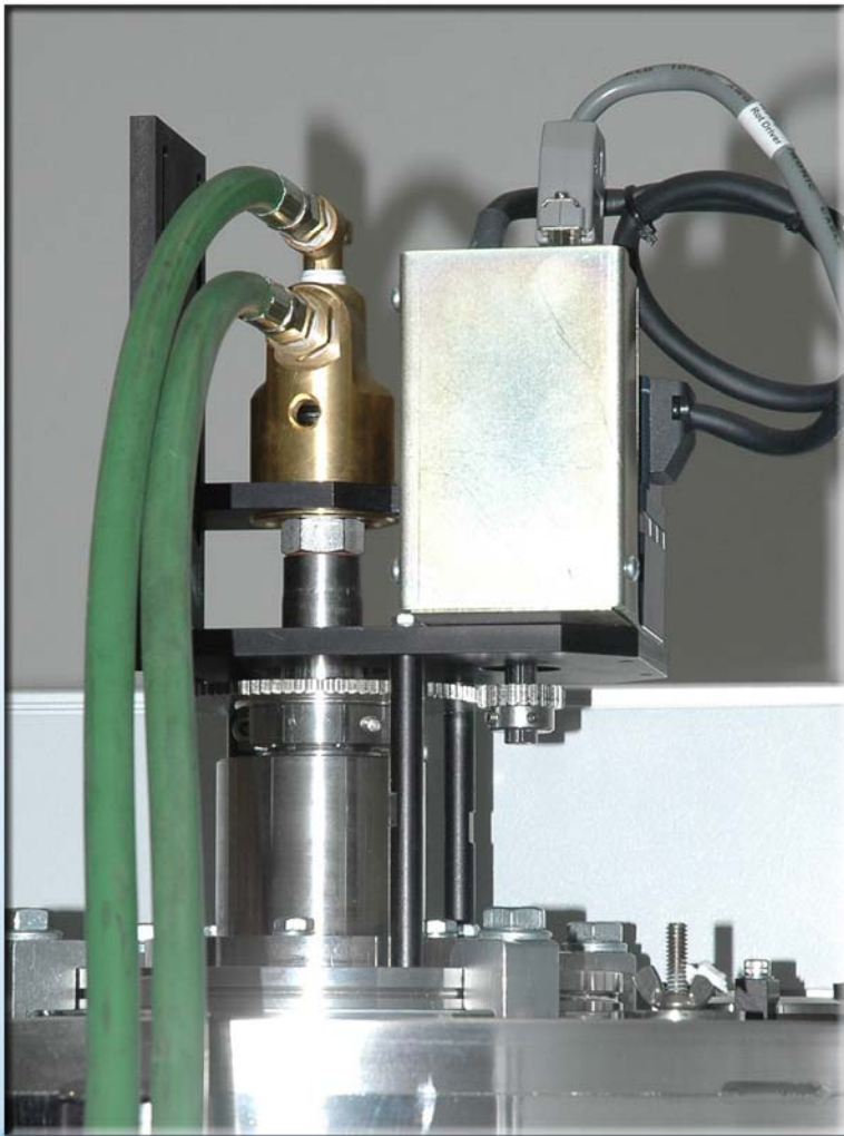
ROTARY UNIT INSTALLED IN THE VACUUM COATER
